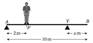
The support B is moved to a point Y on the girder, where BY = x metres, as shown. The man remains on the girder at P. The magnitudes of the reactions at the two supports are now equal.
