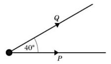
Two forces  $\bf P$  and  $\bf Q$ , act on a particle. The force  $\bf P$  has magnitude 5 N and the force  $\bf Q$  has magnitude 3 N. The angle between the directions of  $\bf P$  and  $\bf Q$  is  $40^{\circ}$ , as shown in the diagram. The resultant of  $\bf P$  and  $\bf Q$  is  $\bf F$ .
