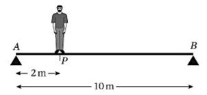
A uniform steel girder AB, of mass 150 kg and length 10 m, rests horizontally on two supports at A and B. A man of mass 90 kg stands on the girder at the point P, where AP = 2 m, as shown. By modelling the girder as a uniform rod and the man as a particle.
