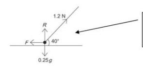
Draw a diagram showing the forces acting on the ring. Include the weight 0.25g, the normal reaction R and the friction force F.
