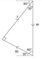
Calculate the angles of the triangle using  $90^{\circ} - 60^{\circ} = 30^{\circ}, 90^{\circ} - 30^{\circ} = 60^{\circ}$  and angles of a triangle add up to  $180^{\circ}$  to give  $90^{\circ}$  as the third angle.
