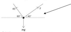
Draw a diagram showing the tension T in the string and the weight mg of the particle.
