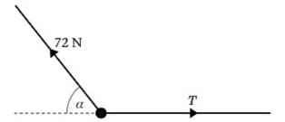
A body of mass 5 kg is held in equilibrium under gravity by two inextensible light ropes. One rope is horizontal, the other is at an angle  $\alpha$  to the horizontal, as shown. The tension in the rope inclined at  $\alpha$  to the horizontal is 72 N. Find
