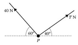
A particle P is held in equilibrium under gravity by two light, inextensible strings. One string is inclined at an angle of  $60^{\circ}$  to the horizontal and has a tension of 40 N. The other string is inclined at an angle of  $40^{\circ}$  to the horizontal and has a tension of T newtons, as shown. Find, to three significant figures,
