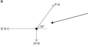
Draw a diagram, showing the weight as well as the tensions in the strings.
