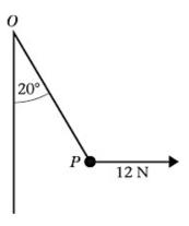
A particle P is attached to one end of a light inextensible string. The other end of the string is attached to a fixed point O. A horizontal force of magnitude 12 N is applied to P. The particle P is in equilibrium with the string taut and OP making an angle of  $20^{\circ}$  with the downward vertical, as shown. Find
