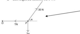
Draw a diagram, showing the weight 2g N as well as the force 30 N and the tension T N.
