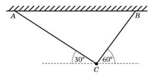
A particle of weight W newtons is attached at C to the ends of two light inextensible strings AC and BC. The other ends of the strings are attached to two fixed points A and B on a horizontal ceiling. The particle hangs in equilibrium with AC and BC inclined to the horizontal at 30° and 60° respectively, as shown. Given the tension in AC is 50 N, calculate
