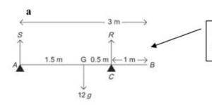
Draw a diagram showing the reactions at the supports and the weight of the beam.
